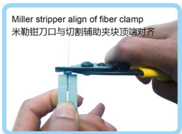
1.3 Press the cable into the clamp
