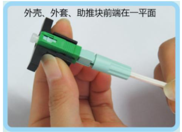
2.4 Lock the fiber(Take off the switch)
